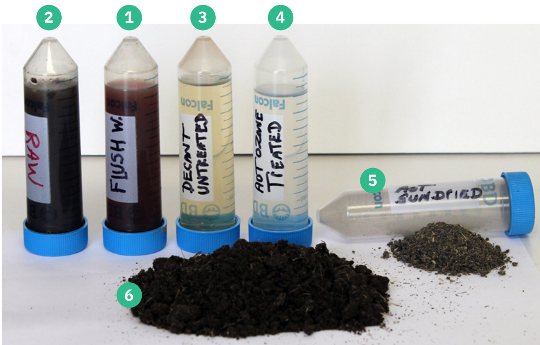
Fig 1. Water & fertilizer samples from traditional waste treatment vs. AOT™ (sample numbers correlate with those on Fig. 2)
